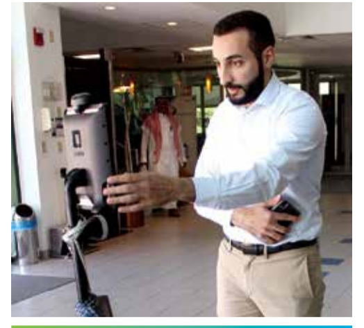
A guest interacts with the Noor robot. Standing about 2 meters tall, Noor consists of a touch screen and a mobile base equipped with motorized wheels. Using advanced telecommunications technology, an operator can effortlessly control Noor from just a few feet, or many miles away.
