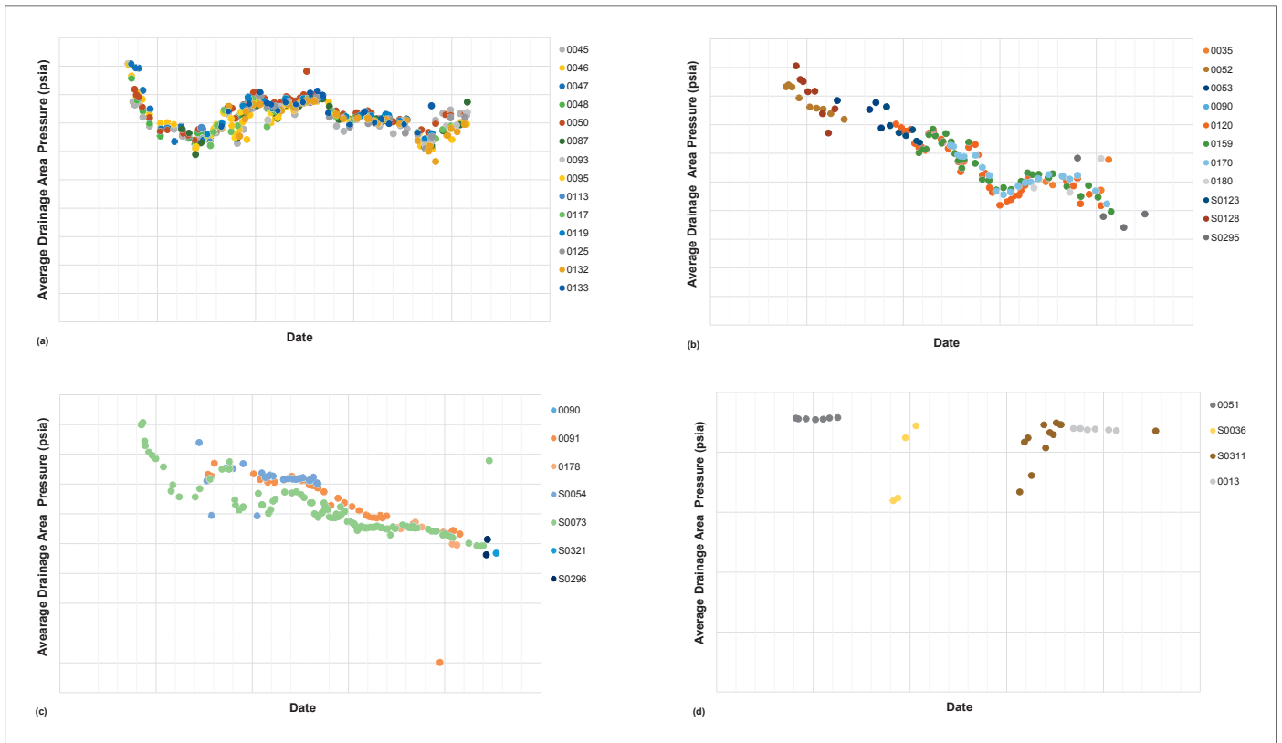
Fig. 17. Four homogeneous pressure groups: (a) CRR-1 wells, (b) CRR-2 wells, (c) CRR-3 wells, and (d) CRR-4 wells, extracted from the globally heterogeneous cloud of shut-in pressures in Res-Y.
