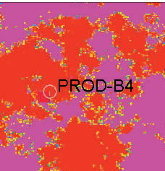
Fig. 10. Prod-B4 low core permeability was captured at the well's location, but the SGS modeling puts high permeability values immediately around the well.
