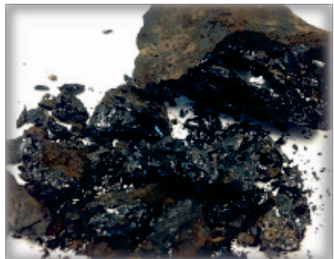
Fig. 1. A bituminous sediment sample (sludge type 1) from an organic rich layer in a sandstone reservoir. The samples have a black vitreous luster with conchoidal fractures. They represent the filling of available porosity because of the thermal conversion of kerogen. Their microscopic appearance reflects the shape of the void they fill.
