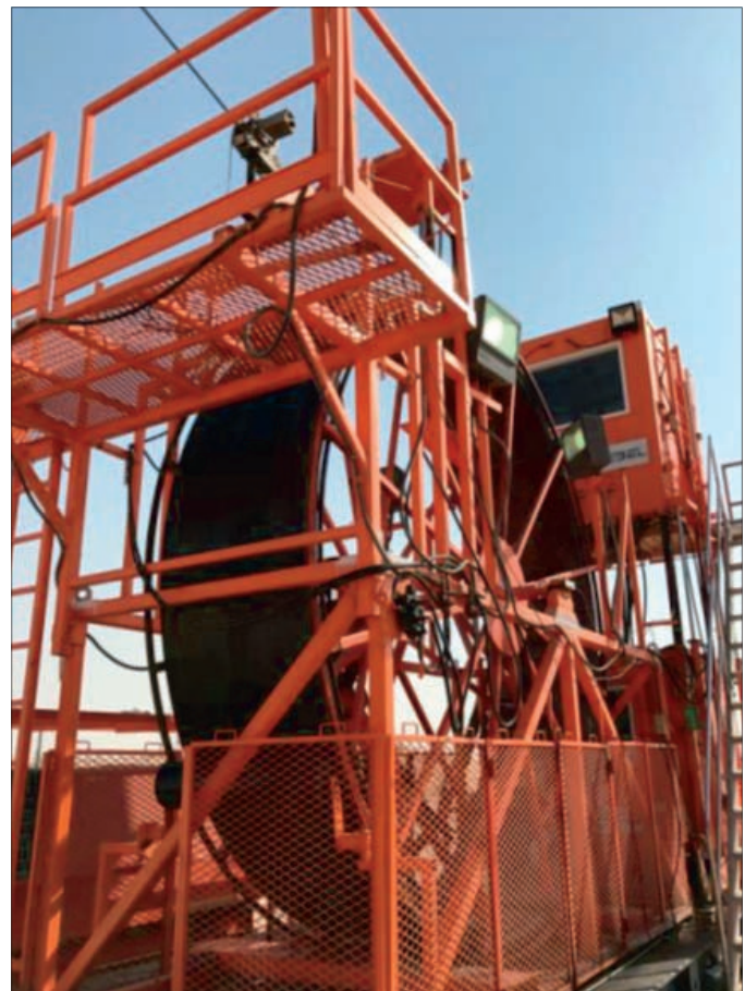
Fig. 3. Carbon rod coiled up on a drum.
