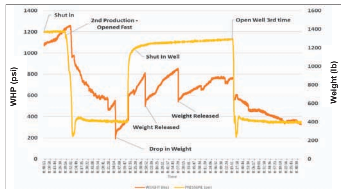
Fig. 7. Carbon rod weight and well flow vs. time for the rest of the sensing sequence.
